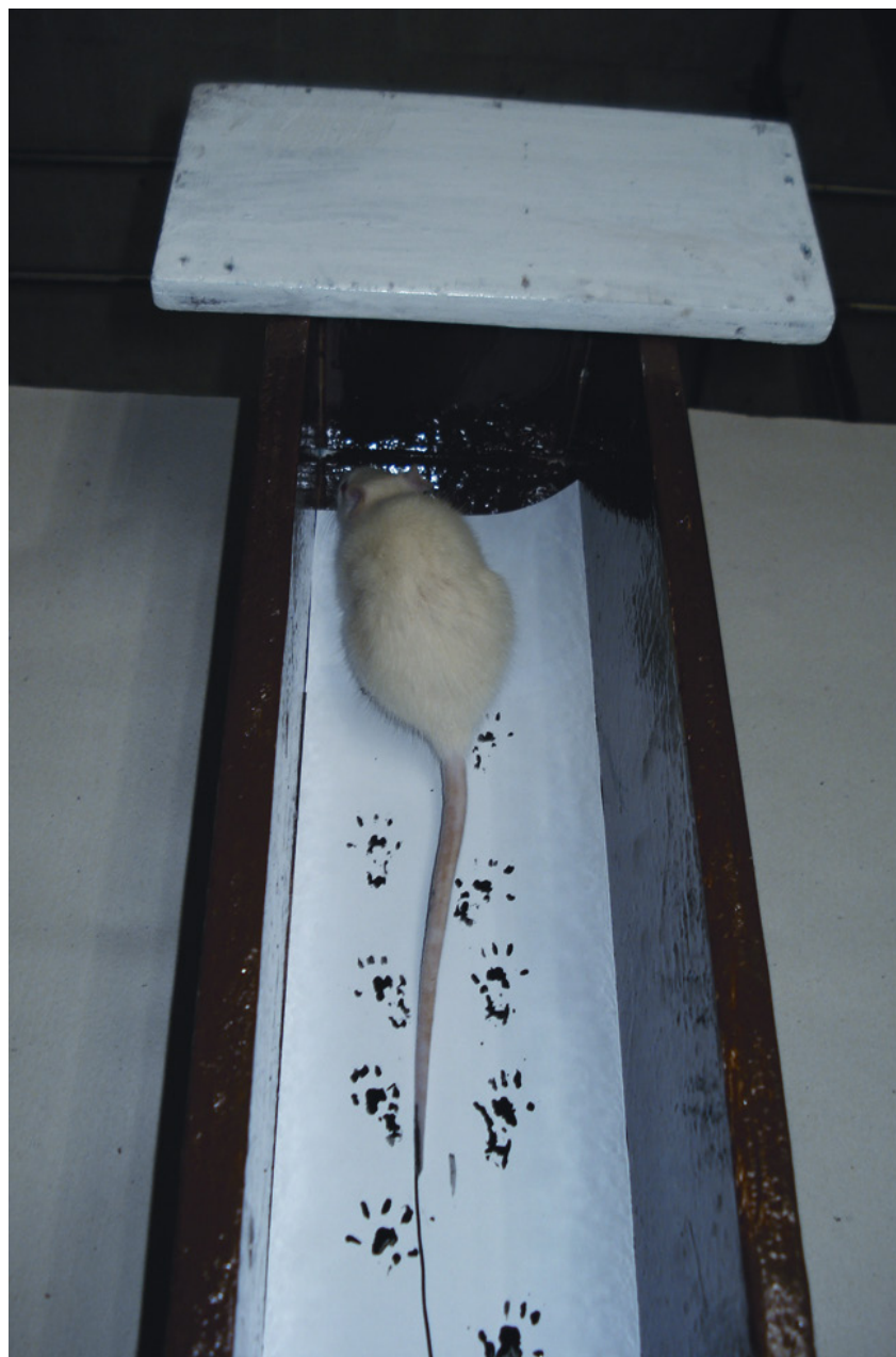
FIGURE 3. Walking track apparatus. Rat in an 8.2 x 42 cm walking track apparatus lined with white office paper. After the hind limbs of the rat are dipped in Chinese ink, the rat walks towards the darkened end of the corridor.
